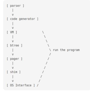
The btree layer and onward is called the storage engine.
